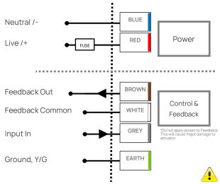
Note that Black is not used as standard unless Alarm Relay option is selected. Separate wiring schematic available for actuators with alarm. For Series 10, you must order the specific Control you require, you cannot select between Control input via firmware as you can with Series 50-400.
