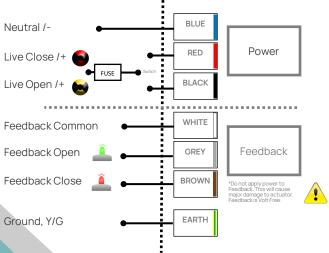
Failsafe versions have internal capacitor, this is charged whilst power is applied. When power is removed, the actuator will close or open depending on what you have ordered. Re-apply power and the capacitor will charge again and is always being charged when power is applied. When actuator is powered, heater is working.
